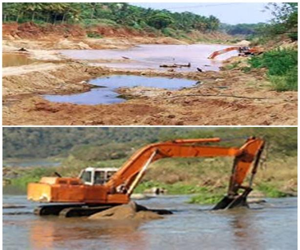
Figure No. 2: River Sand Mining and a Degraded River Bed Source: Coastal Care, 2014.
