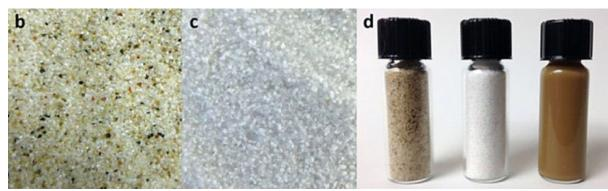
Figure No. 3: Beach sand on the left (b) and purified sand in the middle (c). The right side image (d) shows glass vials containing the former two sand samples, and a third vial containing nano-silicon made of synthetic industrial heated once beach sand which will be used to make the battery.
